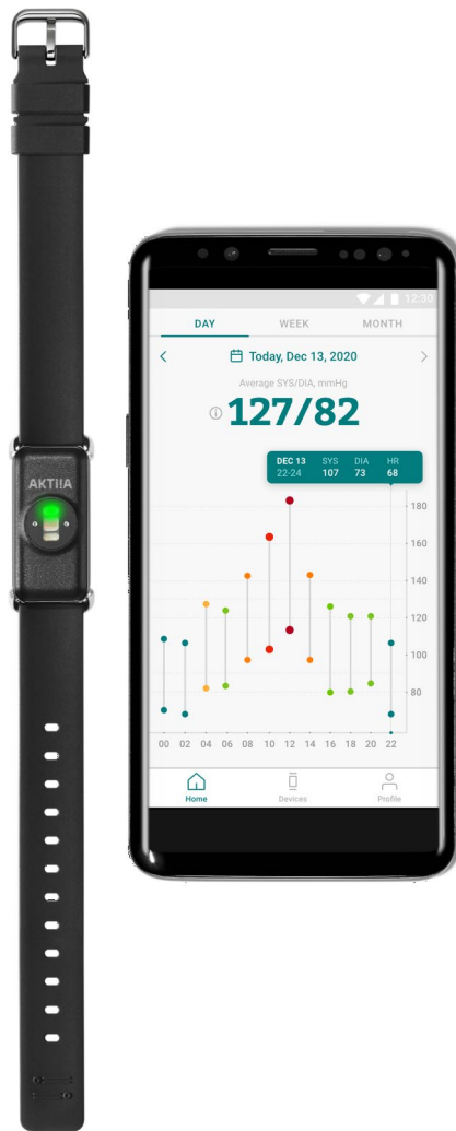
Figure 1. The Aktiia 24/7 BP monitor is a wearable device that persistently measures optical signals on the skin vasculature of the wrist and displays day and night BP values on a companion smartphone application. The Aktiia Bracelet is a CE-marked class IIa medical device.
